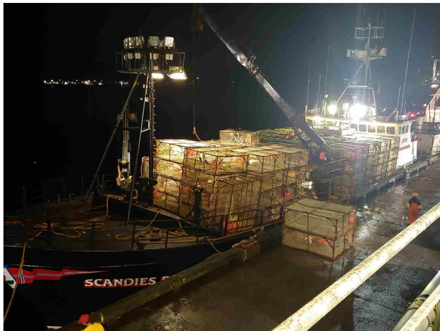
Figure 2: SCANDIES ROSE Crab Pot Loading from Unidentified Voyage. Assumed to be Typical Crab Pot Loading (Provided to MSC by Marine Board of Investigation)
