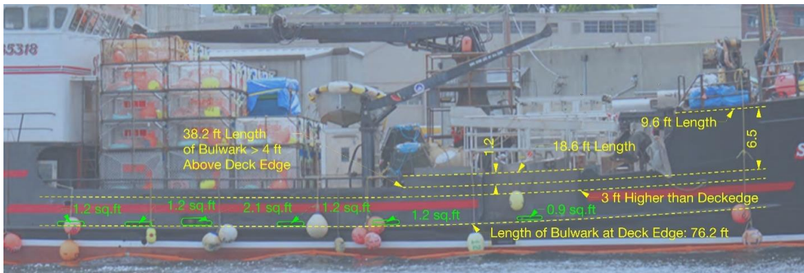
Figure 30: Profile Picture of SCANDIES ROSE from Ref (o) with Scaled Freeing Port Areas and Deck Lengths, the photograph and measurements are scaled with Rhinoceros drawing software
